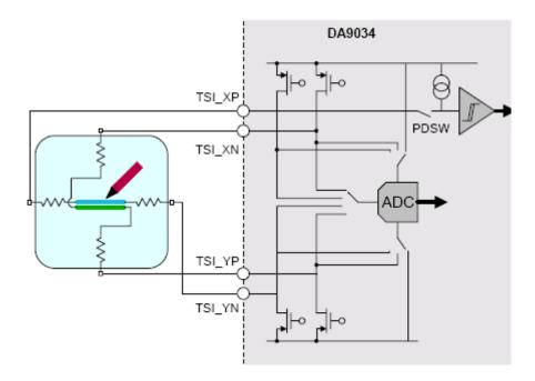
The VAR-SOM-OM35 outputs Touch Screen Controller signals:
